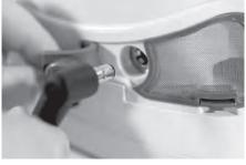
2. Connect the AC power cord to the AC power brick.
